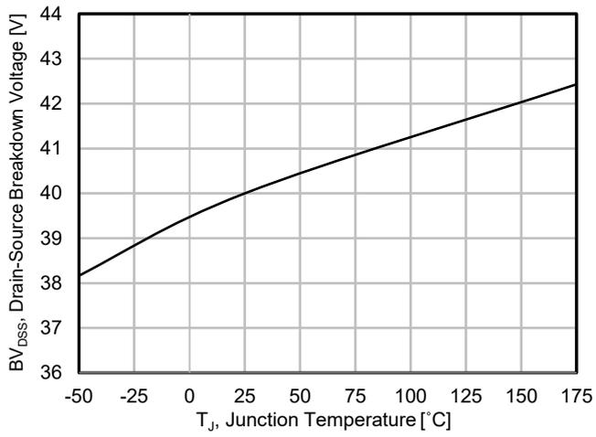
**Fig. 13.  $BV_{DSS}$  Variation with Temperature**
