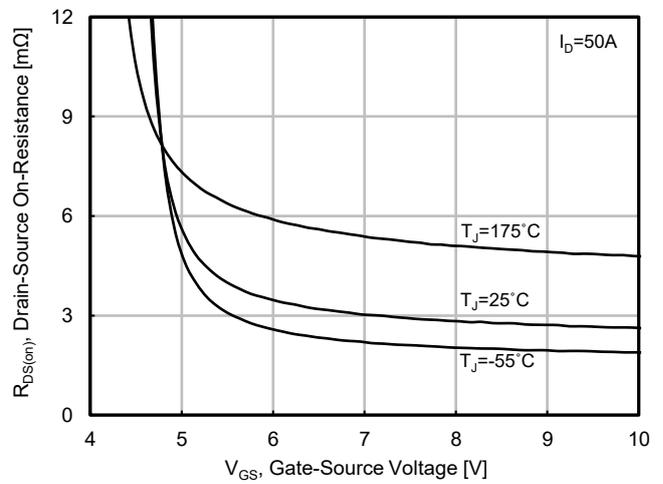
**Fig. 4. On-Resistance vs. Gate to Source Voltage**
