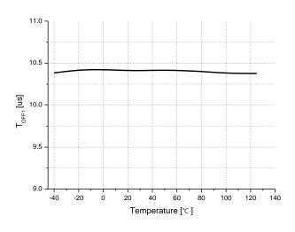
$t_{\text{OFF2}}(R_{\text{TOFF}}\text{=}36k\Omega)$  vs. Temp.
