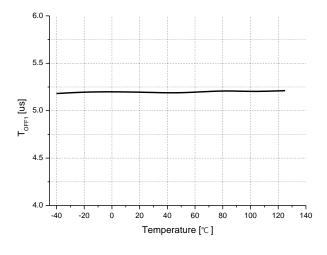
$t_{OFF}(R_{TOFF}=103k\Omega)$  vs. Temp.
