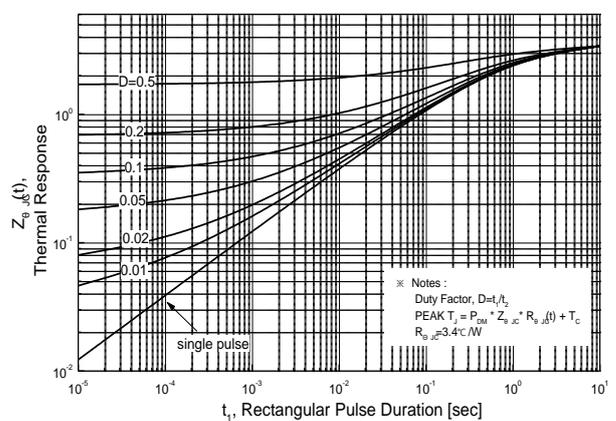
Fig.12 Transient Thermal Response Curve MDF15N60G(TO-220F)
