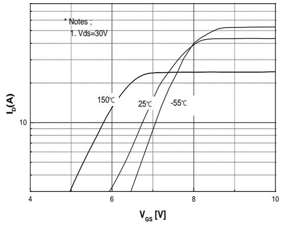
Fig.5 Transfer Characteristics
