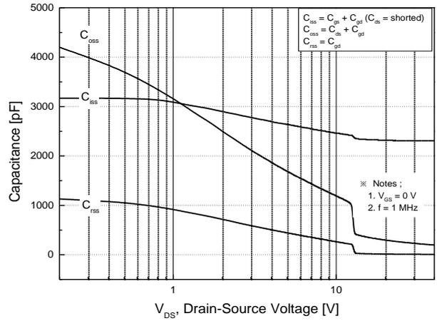
Fig.8 Capacitance Characteristics
