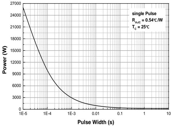
**Fig.13 Single Pulse Maximum Power Dissipation MDP15N60G(TO-220)**
