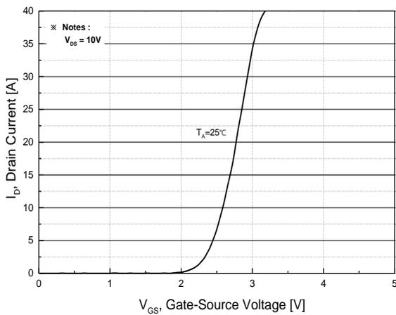
**Fig.5 Transfer Characteristics**
