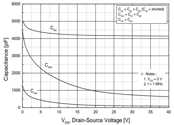
**Fig.8 Capacitance Characteristics**
