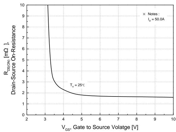
**Fig.4 On-Resistance Variation with Gate to Source Voltage**
