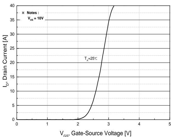
**Fig.5 Transfer Characteristics**
