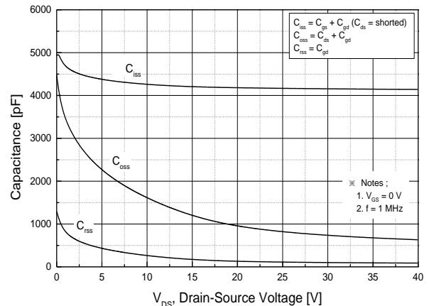
**Fig.8 Capacitance Characteristics**
