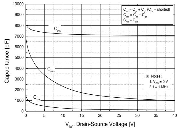
**Fig.8 Capacitance Characteristics**
