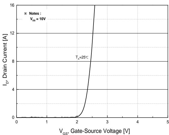
**Fig.5 Transfer Characteristics**
