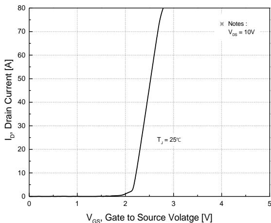
**Fig.5 Transfer Characteristics**
