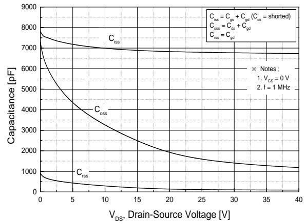
**Fig.8 Capacitance Characteristics**
