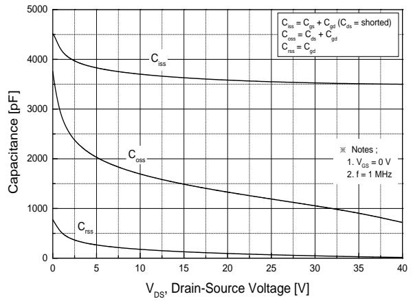
**Fig.8 Capacitance Characteristics**
