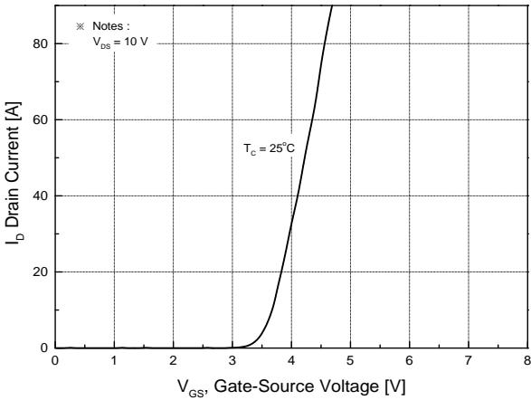
**Fig.5 Transfer Characteristics**
