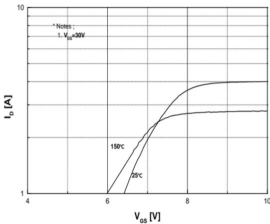
**Fig.5 Transfer Characteristics**
