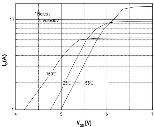
**Fig.5 Transfer Characteristics**
