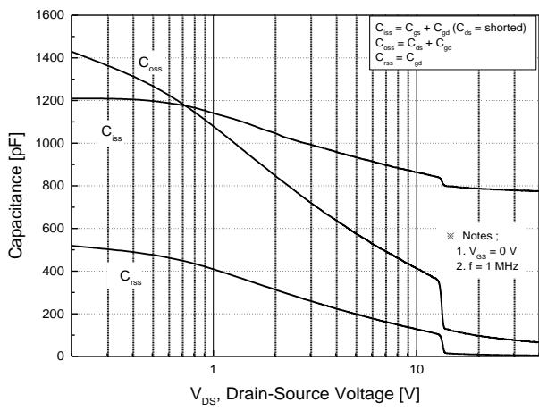
**Fig.8 Capacitance Characteristics**
