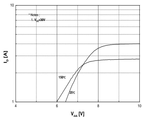
**Fig.5 Transfer Characteristics**
