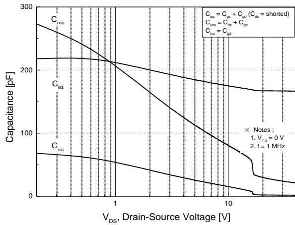
**Fig.8 Capacitance Characteristics**
