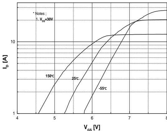
**Fig.5 Transfer Characteristics**
