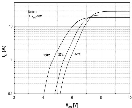
**Fig.5 Transfer Characteristics**
