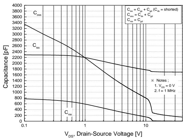
**Fig.8 Capacitance Characteristics**
