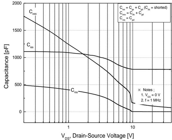
**Fig.8 Capacitance Characteristics**
