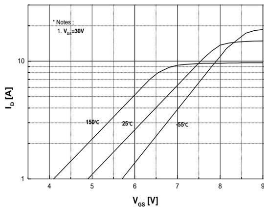
**Fig.5 Transfer Characteristics**
