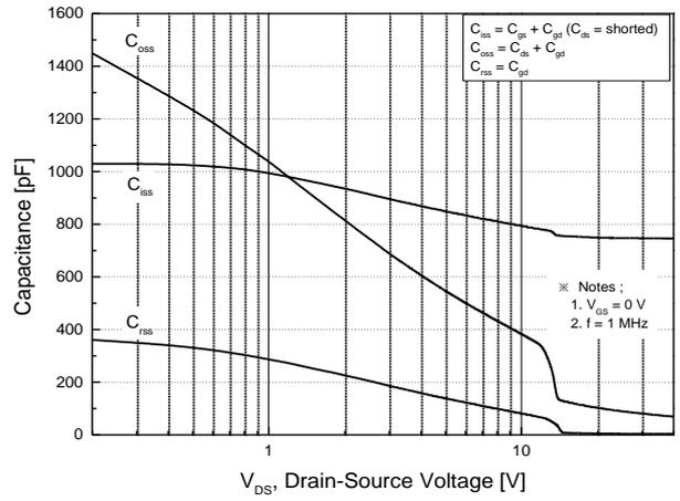
**Fig.8 Capacitance Characteristics**
