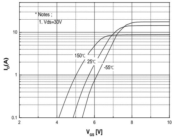
**Fig.5 Transfer Characteristics**
