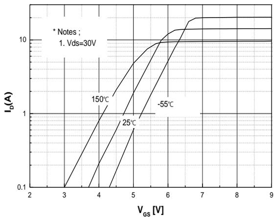
**Fig.5 Transfer Characteristics**
