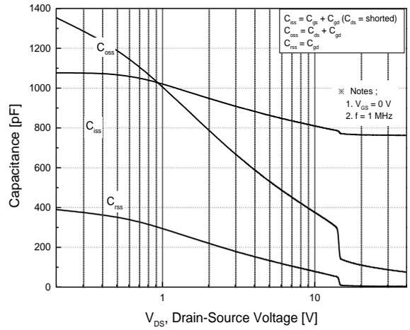
**Fig.8 Capacitance Characteristics**
