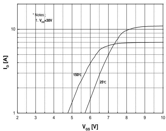
**Fig.5 Transfer Characteristics**
