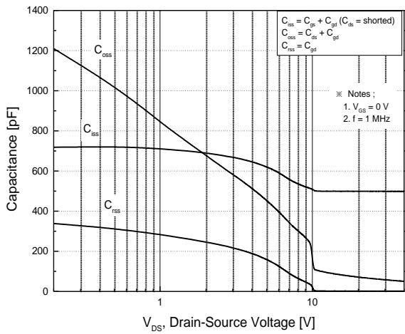
**Fig.8 Capacitance Characteristics**
