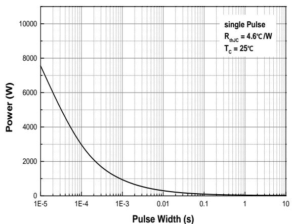
**Fig.12 Single Pulse Maximum Power
