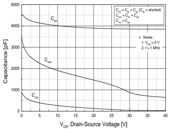
**Fig.8 Capacitance Characteristics**
