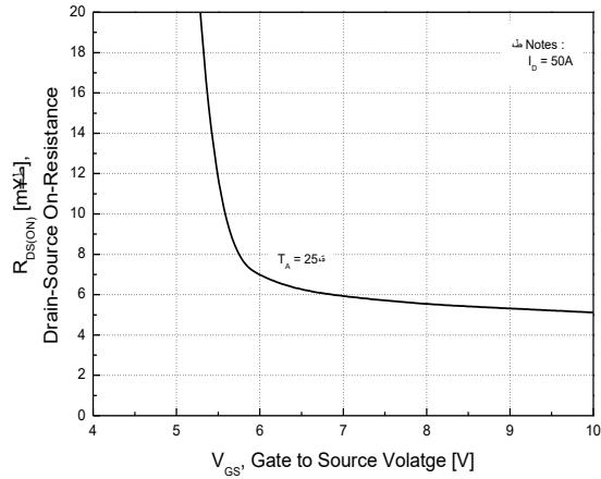
**Fig.4 On-Resistance Variation with Gate to Source Voltage**
