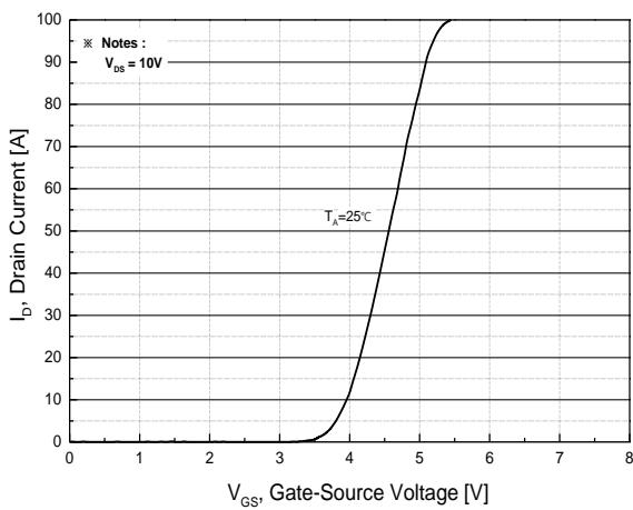
**Fig.5 Transfer Characteristics**
