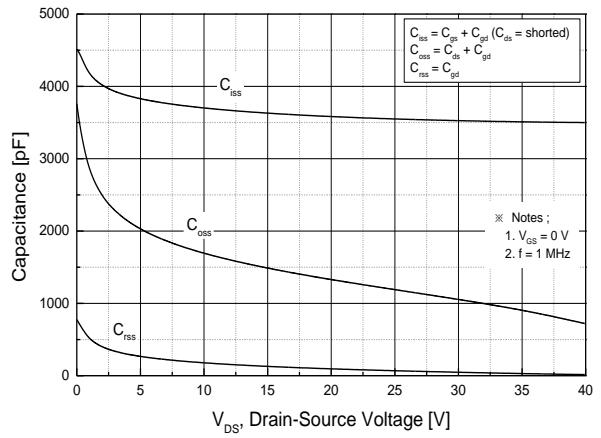
**Fig.8 Capacitance Characteristics**
