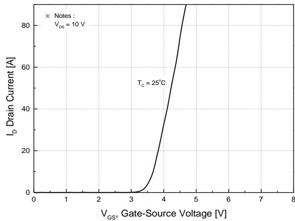
**Fig.5 Transfer Characteristics**
