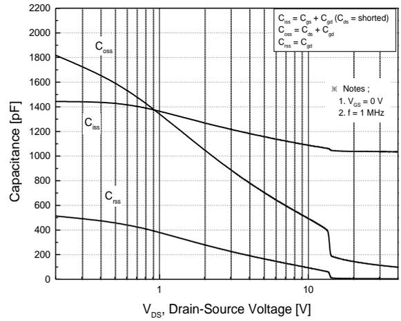
**Fig.8 Capacitance Characteristics**
