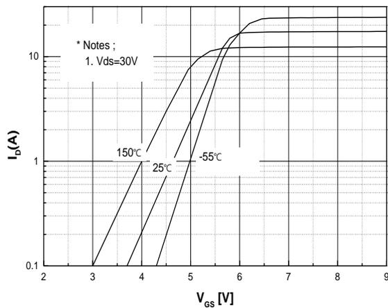
**Fig.5 Transfer Characteristics**
