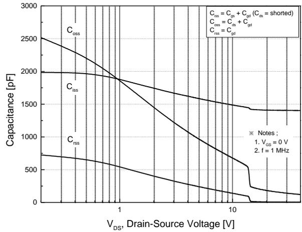
**Fig.8 Capacitance Characteristics**
