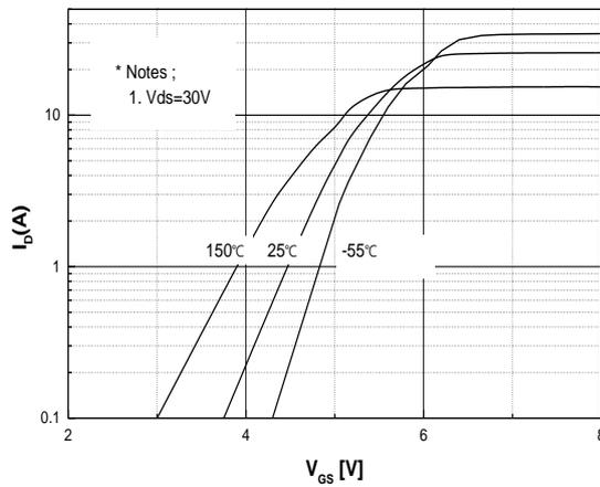
**Fig.5 Transfer Characteristics**
