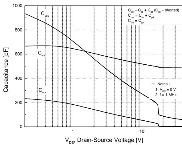
**Fig.8 Capacitance Characteristics**
