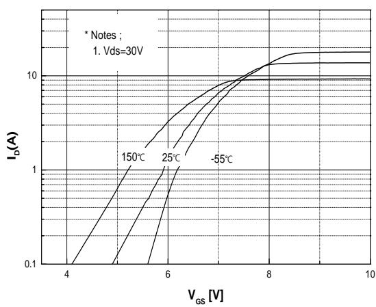
Fig.5 Transfer Characteristics
