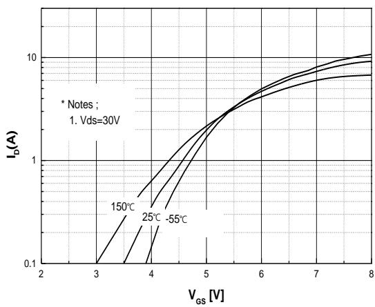
**Fig.5 Transfer Characteristics**
