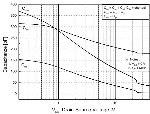
**Fig.8 Capacitance Characteristics**
