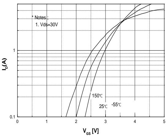
**Fig.5 Transfer Characteristics**
