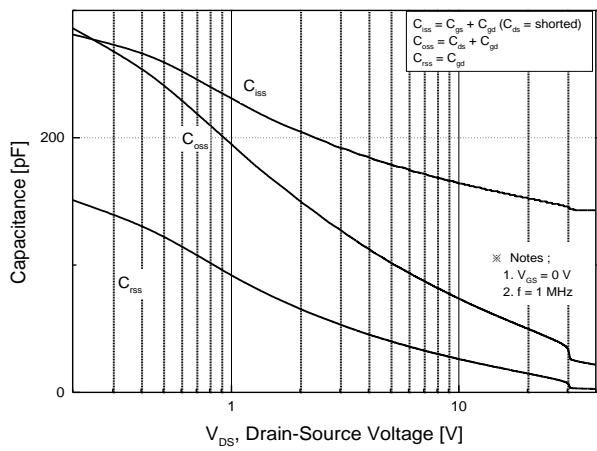
Fig.8 Capacitance Characteristics
