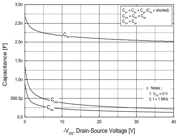
**Fig.8 Capacitance Characteristics**
