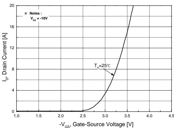
**Fig.5 Transfer Characteristics**
