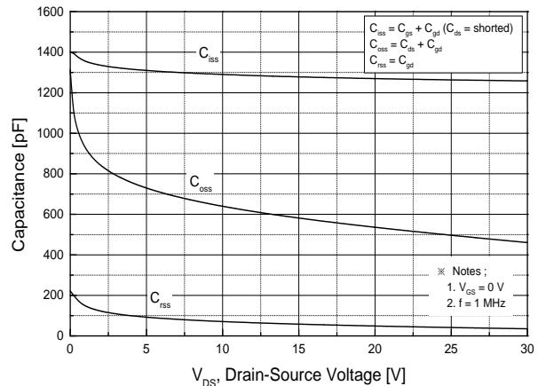
**Fig.8 Capacitance Characteristics**
