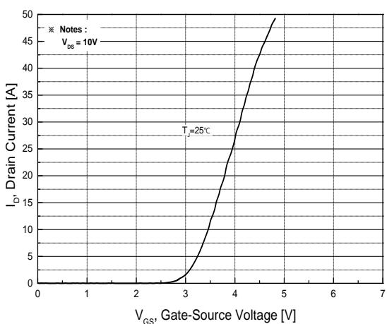
**Fig.5 Transfer Characteristics**
